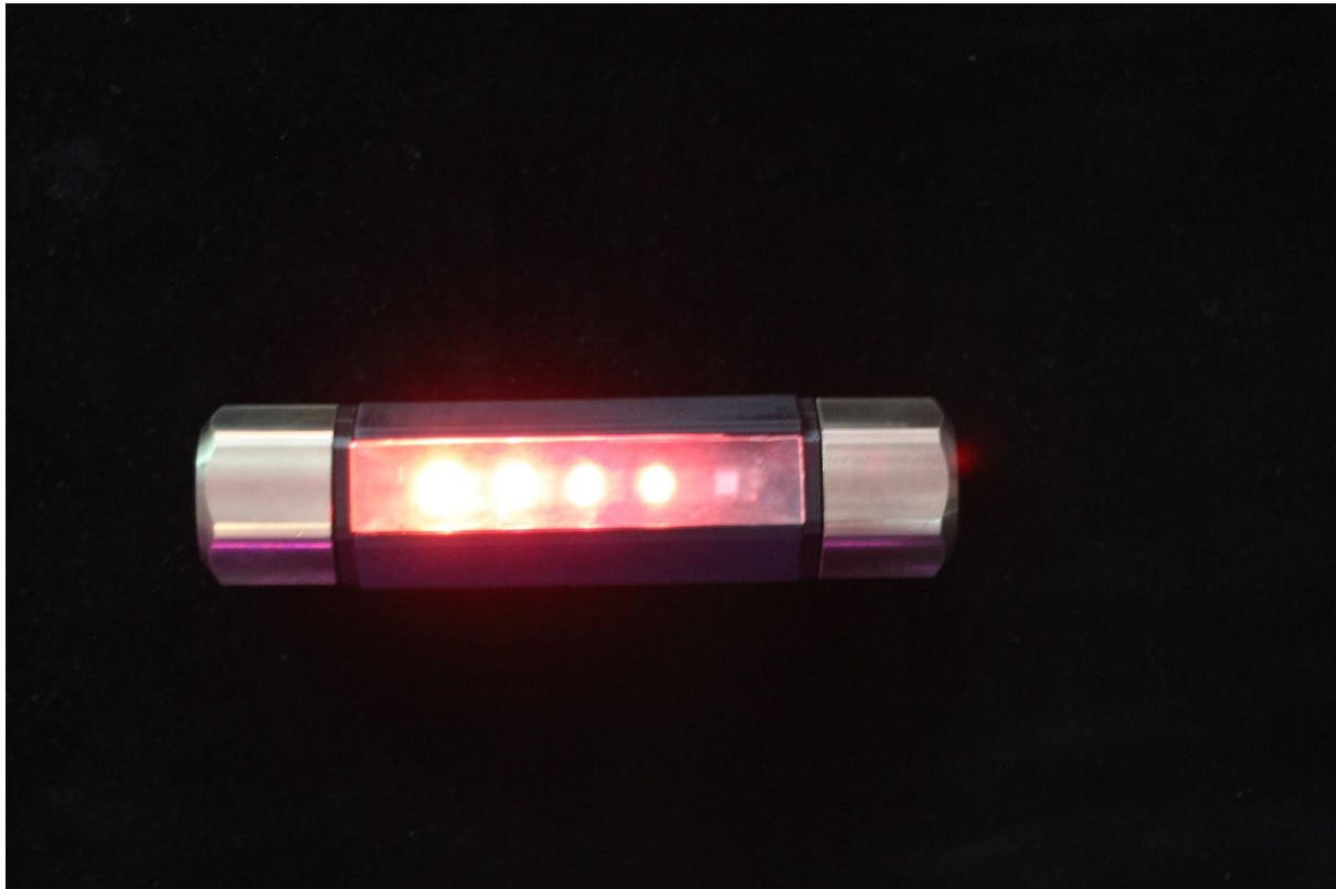
Figure 32: Despite the issues with gluing the acrylic in place, the end result was still a satisfying diffusion of the LED's, particularly for a piece only 1.25mm thick.
