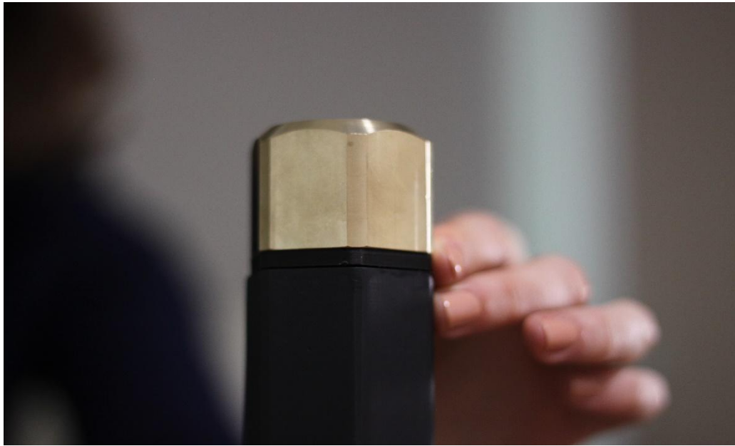
Figure 31: The careful measurements and checks paid off – when the brass was complete, each fit perfectly flush against the edge of the concept prototype body.
