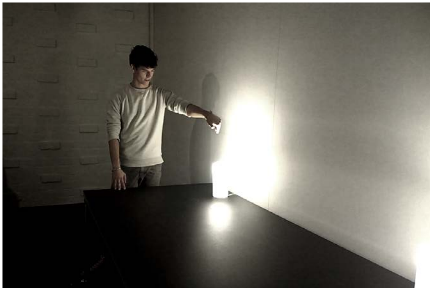
Figure 4: impression of the first part of the user test where the participant was asked to control the light without any controlling devices. This picture shows an example of a gesture to change the brightness of the lamp.
